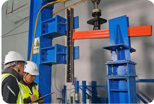
Beam End Tab Testing
