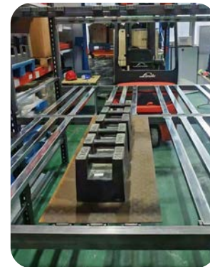
Cross Beam Load Testing
